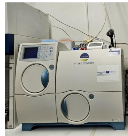
Vitek 2 automated platform for microbial identification and antimicrobial susceptibility testing
